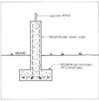
Figure 4.19. Reinforced Concrete Pier
