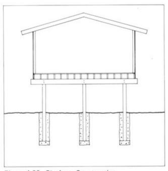
Figure 4.28. Platform Construction
