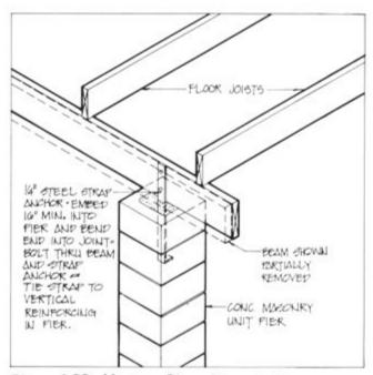
Figure 4.36. Masonry Pier-Strap Anchor
