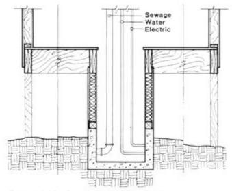
Figure 4.48. Protective Utility Shaft
