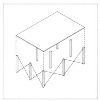
Figure 4.22. Diagonal Bracing
