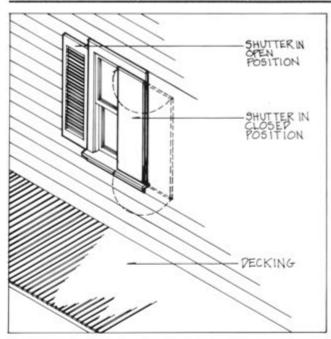
Figure 4.47. Shutters for Window Protection
