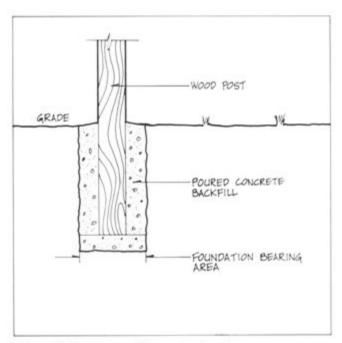
Figure 4.7. Post on Concrete Bearing Pad
