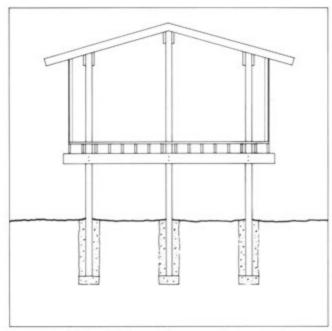
Figure 4.29, Pole Frame Construction
