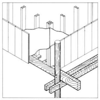
Figure 4.30. Exterior Pole Framing
