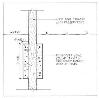
Figure 4.5. Reinforced Concrete Collar
