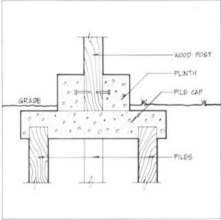
Figure 4.8. Post/Pile Foundation
