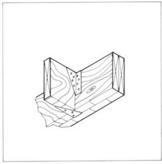
Figure 4.27. Metal Framing Anchors
