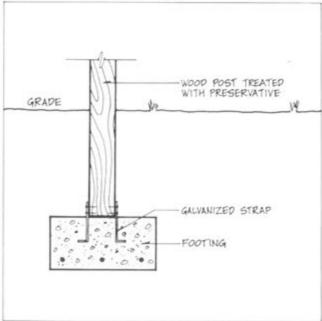
Figure 4.13. Galvanized Strap Anchorage Detail
