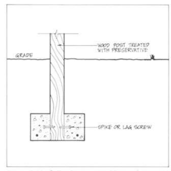
Figure 4.11. Spike Anchorage of Post
