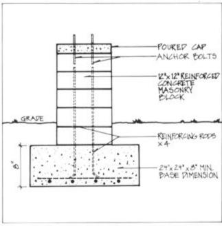
Figure 4.17. Reinforced Concrete Masonry Pier
