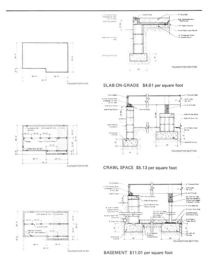
Figure 5.1. Conventional Foundations (Estimates are spring 1983.)
