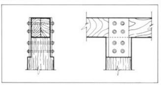
Figure 4.32. Dapped Gusset Plate Connection
