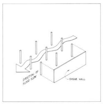
Figure 4.24. Shear Wall Bracing
