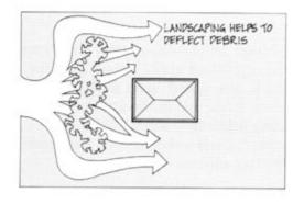
Figure 2.6. Site Design to Reduce Flood Hazards
