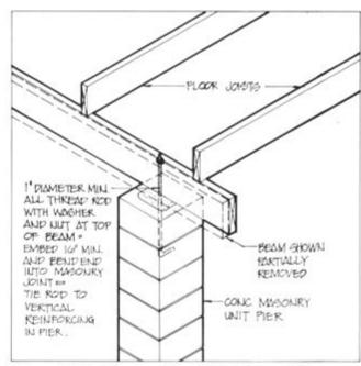
Figure 4.37. Masonry Pier-Bolt Through Beam
