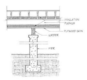
Figure 4.53. Double-Insulated Floor Plenum, Pier Foundation
