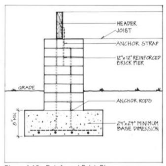
Figure 4.16. Reinforced Brick Pier
