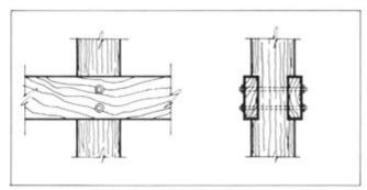
Figure 4.33. Dapped Pole Connection
