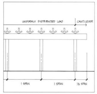
Figure 4.39. Floor Beam with Cantilever Overhang
