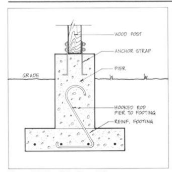
Figure 4.9. Post/Pier Foundation
