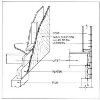
Figure 4.45. Plywood Anchorage
