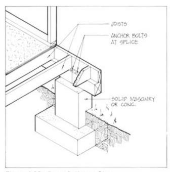
Figure 4.38. Beam Splice on Pier
