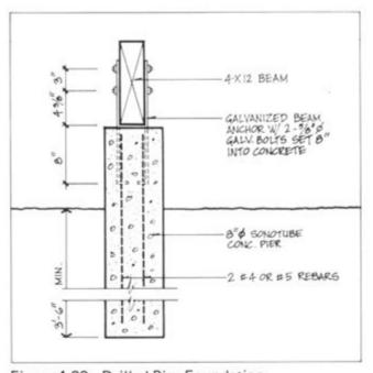
Figure 4.20. Drilled Pier Foundation
