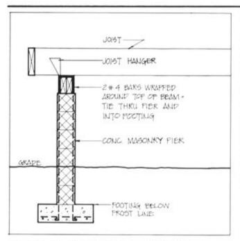
Figure 4.35. Concrete Masonry Unit Pier
