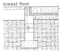
Figure 1.3. Elevation Requirements for Slab Foundations
