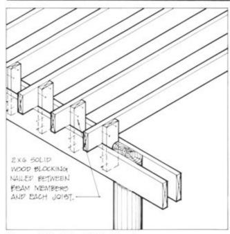
Figure 4.41. Wood Joist Anchors
