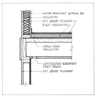
Figure 4.52. Insulated Floor Section, Foundation Wall
