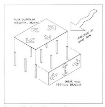
Figure 4.25. Floor Diaphragm Bracing
