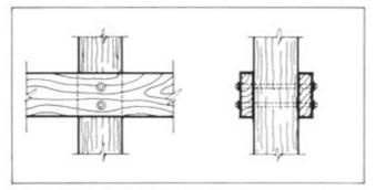
Figure 4.31. Bolted Connection to Round Pole
